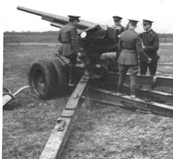
Figure 8: T3 gun mount in 90 degree firing mode. The split trail setup allowed for greater traverse and tube elevation than a box trail setup allowed. G.M. Barnes, "Division Artillery in the Next War" The Field Artillery Journal , Frontispiece.
